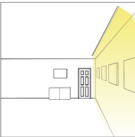
WALL WASH DIRECTION OF LIGHT SHOWN WITH 10 WATT, 3000K VERSION
