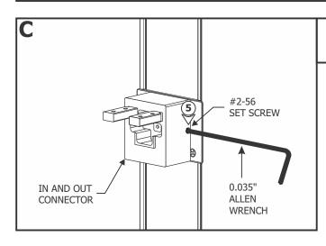
**5:** Place the connector on the mounting plate and secure it in place by tightening the two #2-56 set screws with a 0.035 Allen wrench.
