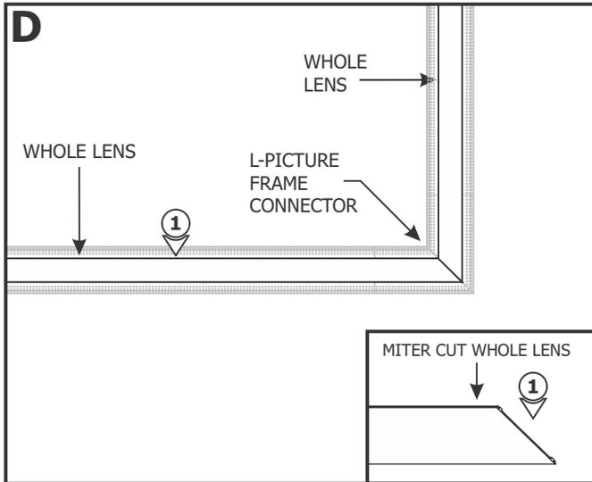
**1:** To avoid seams and light leaks, use the precut lenses that were provided with the L-Picture Frame Connector as a guide to miter cut the whole lenses. Use the whole lenses to cover the L-Picture Frame Connector along with the rest of the installed channels.
