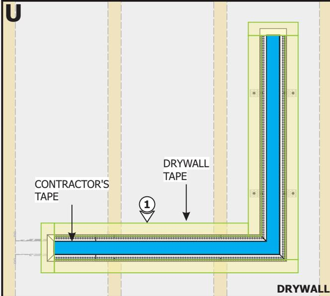
**NOTE:** Cover the channel opening with contractor's tape before plastering.
