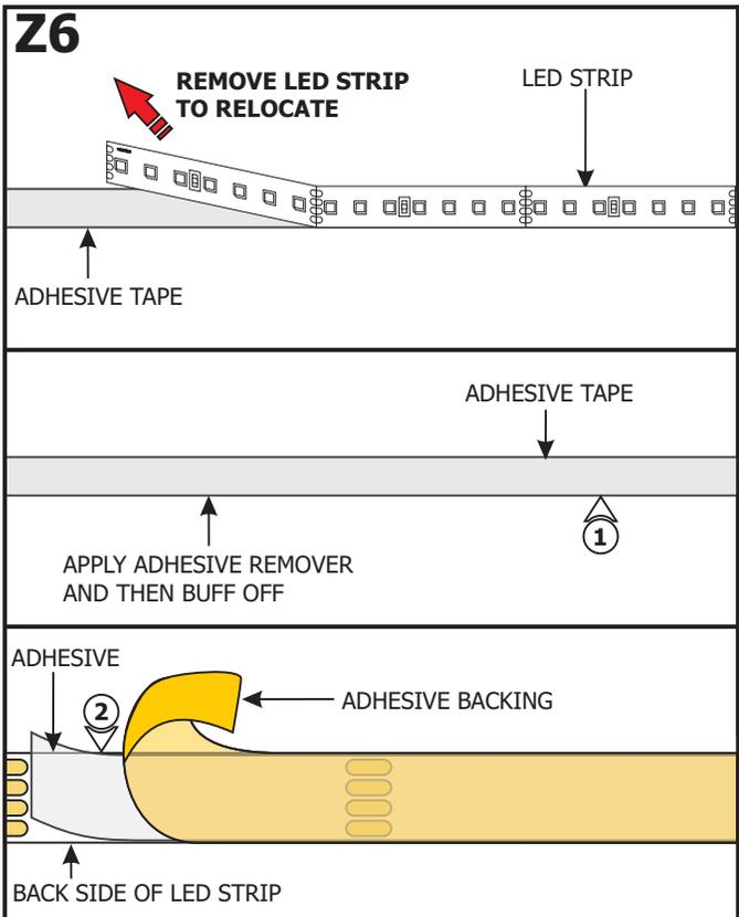
**NOTE:** If relocating the installed LED strip, make sure that the adhesive tape on back of the LED strip covers the entire strip. The adhesive tape isolates the strip from the installation surface. Damaged or inconsistent adhesive tape may cause the contacts on the back of the strip to come in contact with the conductive heat sink which will cause the strip to short and burn. Call PureEdge Lighting to get replacement adhesive tape and/or optional aluminum heat sink tape (SS-HR-F).
