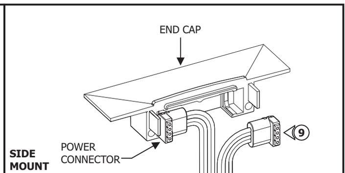
**8: For installations where the LED strip will be laid on the **bottom** of the channel**, place the power connectors into the end cap insert. Slide the end cap insert and power connectors into the end cap.
