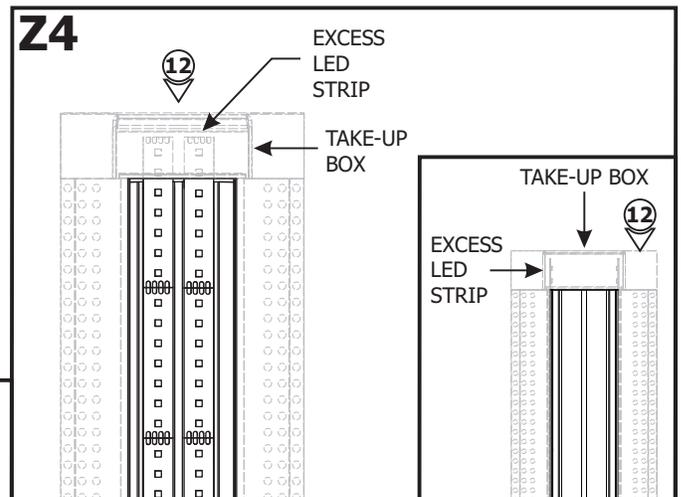
**12:** If required, trim the LED strips on the dashed cuttable section, place the excess LED strips inside the Take-Up Box. Ensure the entire length of the channel is covered with LED strips to avoid unlit areas.
