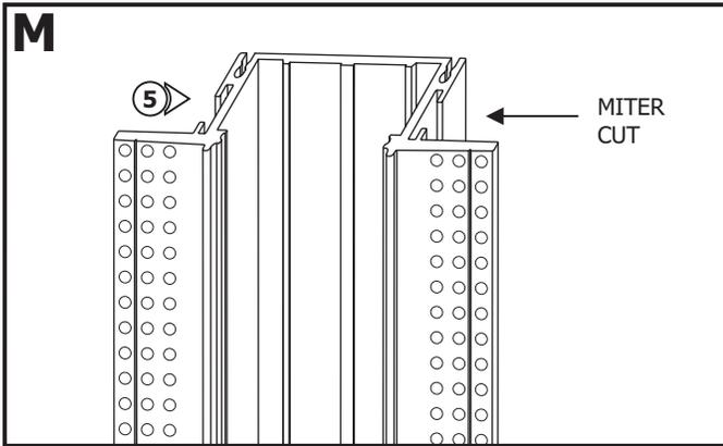
**5: For Room Wrapping Configurations**, miter cut each section of assembled channel and lens to match the corner angle. In a 90° inside corner installation as shown, each channel section is cut at a 45° angle to form a complete corner.
