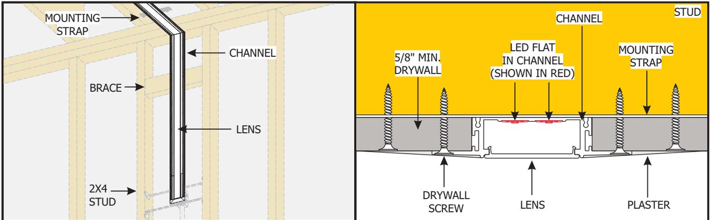
Room-wrapping configurations are used for installations that join runs of **TruLine 1.6A** on multiple planes (like a ceiling and a wall) using miter-cut sections of channel.
