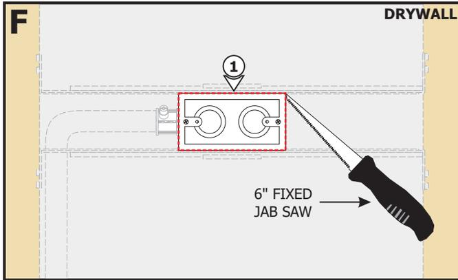
**1:** Cut a section of drywall using a 6" fixed jab saw or other appropriate tool to expose the mounting plate area. Install the drywall.
