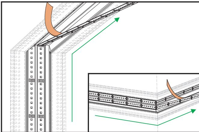
Room-wrapping installations use LED strip bent 90° for inside or outside corner configurations. Channel sections will be miter cut on-site.
