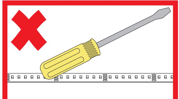
**DO** only ever use fingers to gently install soft strip to a surface **AFTER** cleaning the surface with alcohol.
