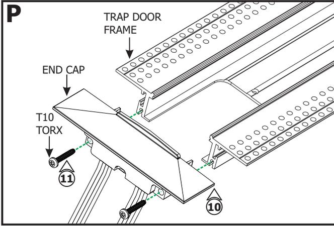
**10:** Insert the #4-40 Torx screws through the end cap holes and thread into the TruLine 1.6A channel.
