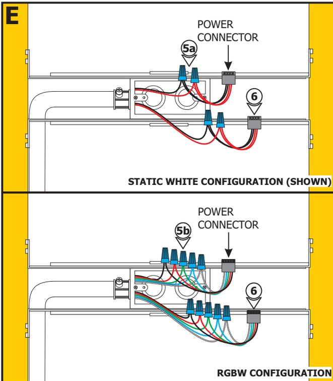
**NOTE:** Remote power supply wires must be present in junction box. Refer to instructions provided with power supply.
