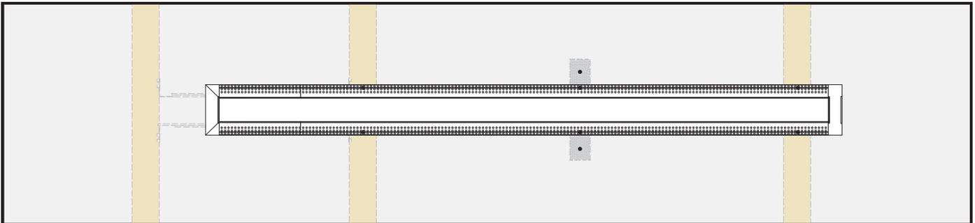
Horizontal installations are linear runs of channel beginning and ending at an end cap and junction/take-up box on a single plane surface. Runs can be up to 40' in length and the LED strip lays in the **bottom** of the channel.
