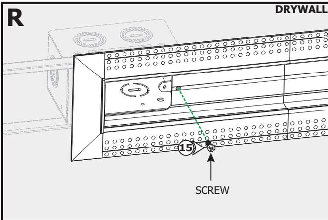
**14:** Place the assembled channel to the cutout area on the wall making sure to fully seat it against the power connector end cap.
