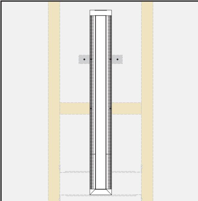
Vertical installations are linear runs of channel beginning and ending at an end cap and junction/take-up box on a single plane surface. Runs can be up to 40' in length and the LED strip lays in the **bottom** of the channel.
