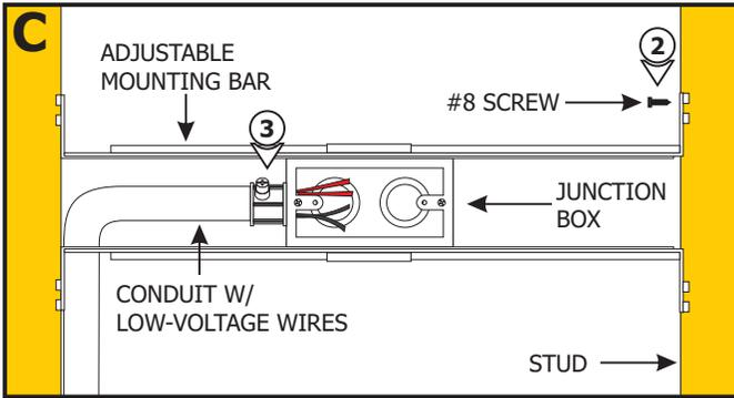
**NOTE:** The adjustable mounting bars mount to studs that are spaced 15" to 24" apart. If the span needs to be shorter than 15", then break the bar arms from dedicated lines.
