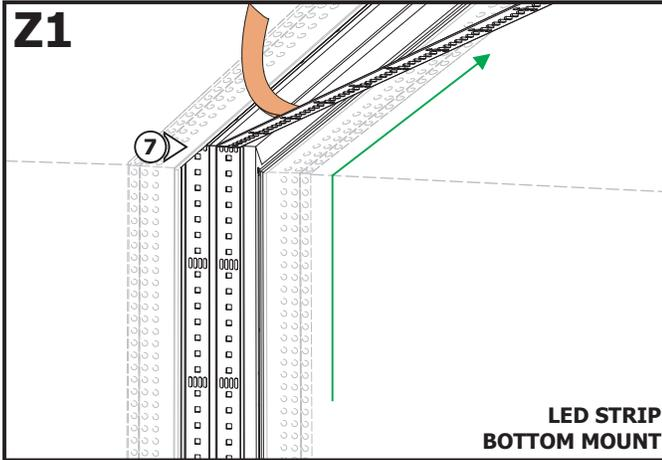
**7: For Room Wrapping Configurations,** bend the LED Strips 90° on the **bottom** of the channel to match the corners. Continue removing the paper backing from the LED strip and installing along channel, pressing adhesive into place using **ONLY** fingers.
