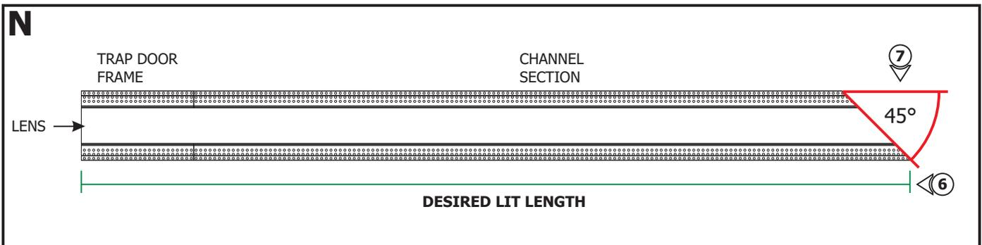
**6: For Zig Zag Configurations**, determine the channel length and cut channel and lens at a 45° angle from the outer corner.
