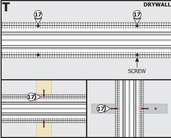
**17:** Properly secure the channel to the marked studs and mounting straps using drywall screws (**DO NOT over tighten**). Ensure all screw heads are flush with the channel surface.
