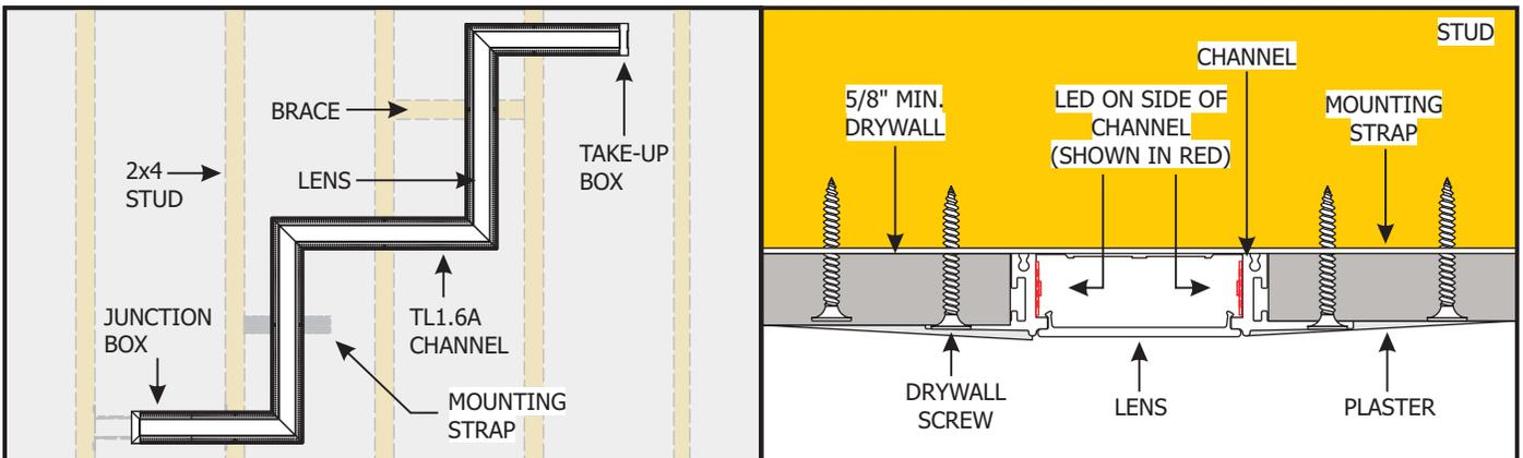
Zig Zag configurations are used for installations that join runs of **TruLine 1.6A** on a single plane (like a ceiling or a wall) using miter-cut sections of channel.
