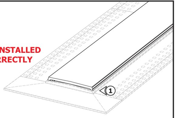
1: Snap the lens back onto the channel. Ensure lens is fully seated.
