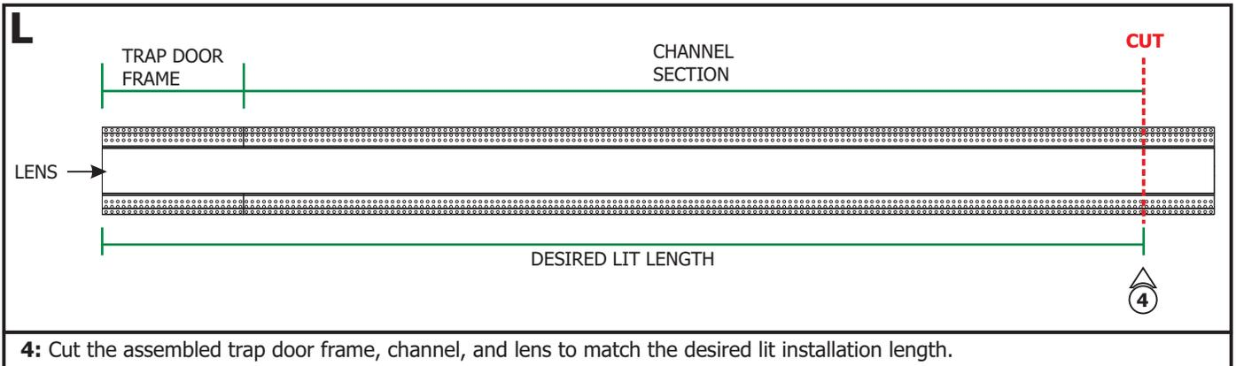
**4:** Cut the assembled trap door frame, channel, and lens to match the desired lit installation length.
