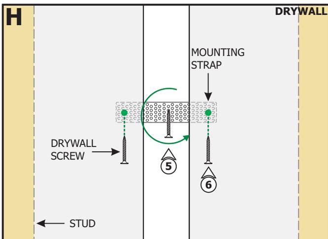
**NOTE:** To install channel in a wall without standard-spaced studs, install perforated mounting straps every 32" behind drywall and secure using two drywall screws. Mark the location of any mounting straps to the drywall (see steps below).
