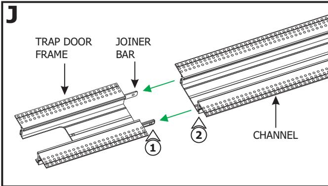
**1:** Insert the joiner bars halfway into the channel trap door frame. Tighten the two M3 set screws on each joiner bar using a 1.5mm Allen wrench.
