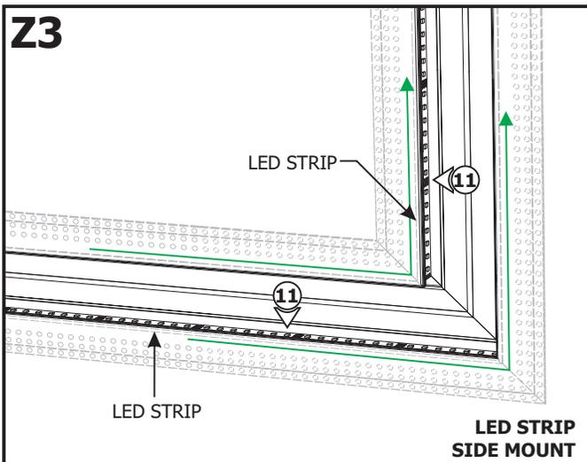
**11: For Zig Zag Configurations,** bend the LED Strips 90° on the **sides** of the channel to match the installation corner. Continue removing the paper backing from the LED strip and installing along channel, pressing adhesive into place using **ONLY** fingers.
