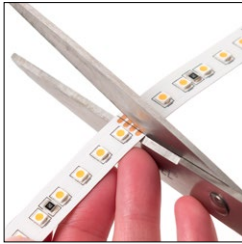
Cut in middle of joining contacts
