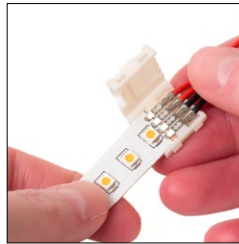
Place the Strip end under the plastic guide and push under the snap contacts.
