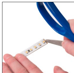
Scrape protective coating from contacts
