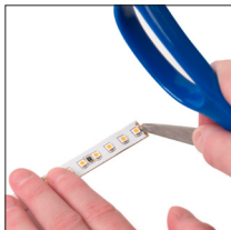
Scrape protective coating from contacts
