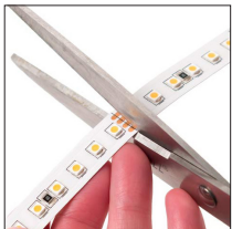
Cut in middle of joining contacts
