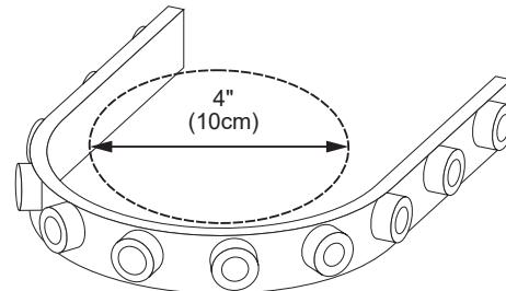
**Drawings:** Dimensions for 2D Flex Lens
