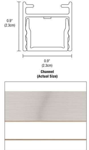
**Drawings:** Dimensions for the Cirrus MIYO Rectangle LED Suspension Lit Corners, Center Feed
