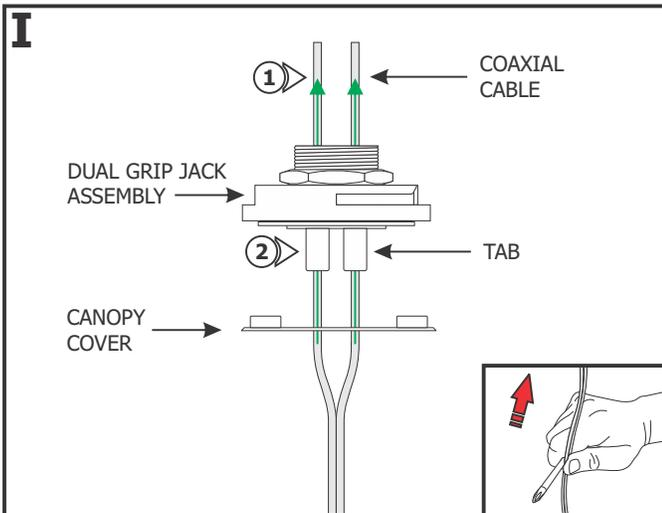
**NOTE:** If cable is curled or kinked, straighten by holding between the shaft of a screwdriver and thumb and pulling the cable through.
