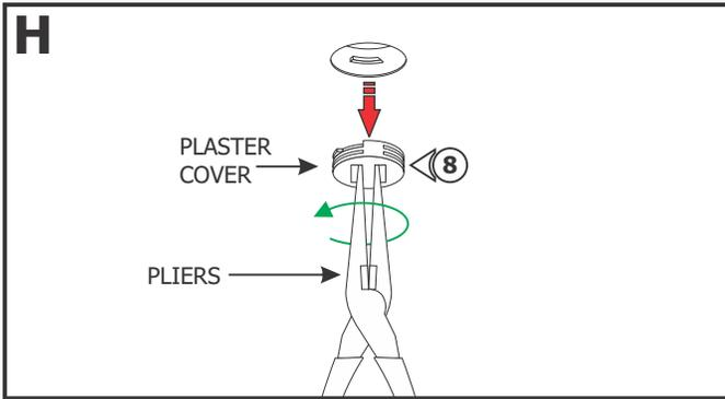
**8:** Use pliers to rotate the plaster cover counter clockwise and remove it. Clean the hole.
