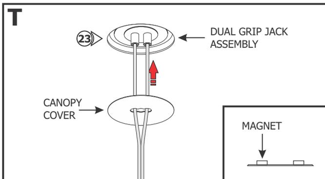
**23:** Place the canopy cover over the Dual Grip Jack assembly. The magnets on the back will keep the canopy cover in place.
