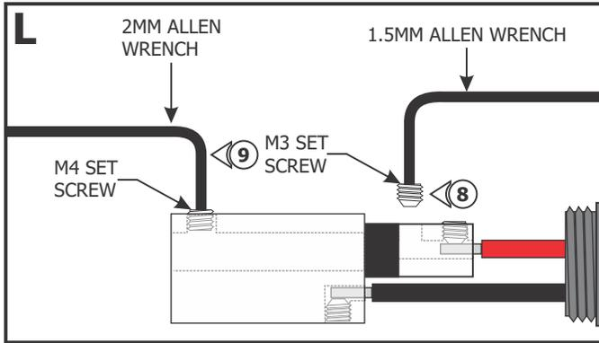
**8:** Using the provided 1.5mm Allen wrench, remove the M3 set screw from the coaxial connector assembly.
