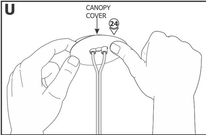
**24:** If necessary, use fingers to push on the perimeter of the canopy cover until it slightly rocks and lift the cover to remove it from the assembly.
