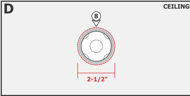
**8:** Use a 2-1/2" hole saw to cut out the drywall section where the junction box opening is located.
