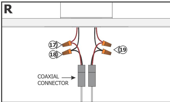
**17:** Connect the +24VDC power supply wire to the red coaxial connector wire using a wire nut.
