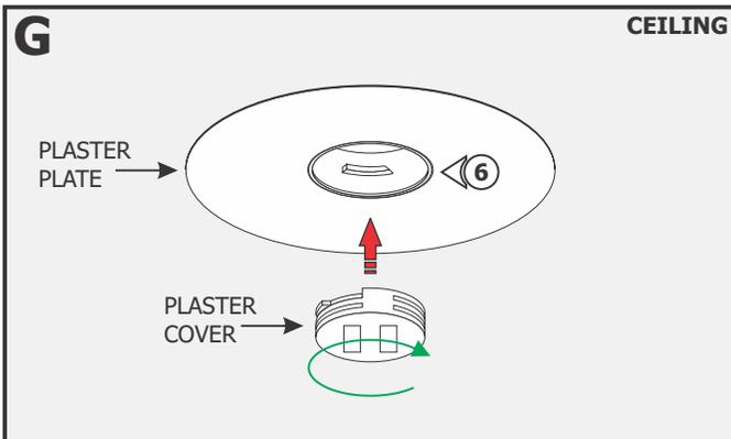
**6:** Rotate the plaster cover clockwise into the plaster plate.
