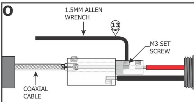
**13:** Use the provided 1.5mm Allen wrench to replace and securely tighten the M3 set screw.
