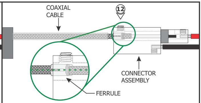
**12:** Insert the coaxial cable into the coaxial connector until the wires of the center conductor are visible through the M3 set screw hole.
