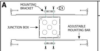
**NOTE:** Adjustable mounting bars mount to studs that are spaced 14.5" to 25" apart.
