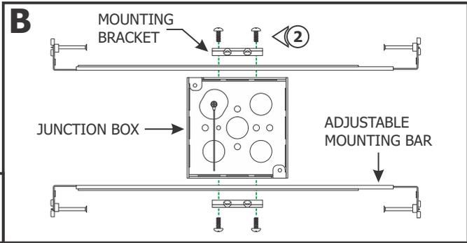
**2:** Mount each adjustable mounting bar to one side of the junction box and secure them with the mounting brackets and two Phillips screws provided.
