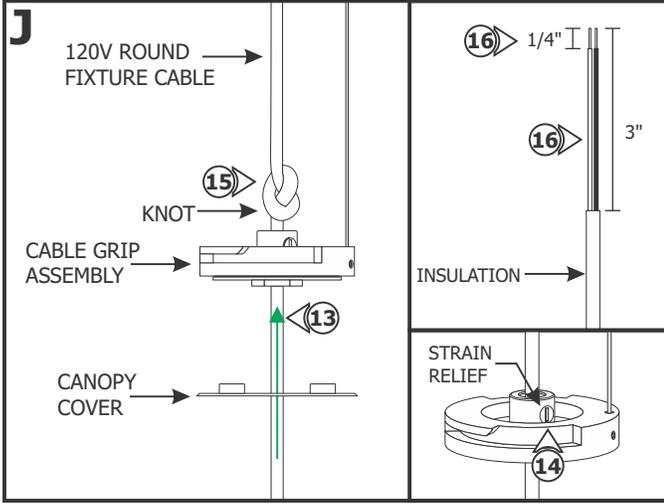
**13:** Feed the 120V round fixture cable (max. 1/4" thick) through the canopy cover and Cable Grip Assembly.
