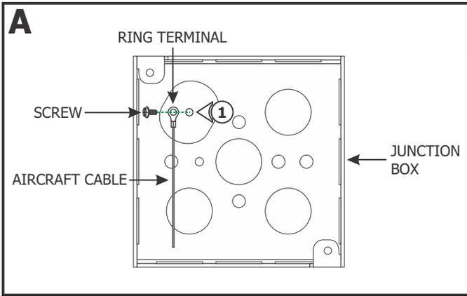
**1:** Attach the ring terminal with aircraft cable to the junction box using the screw provided.
