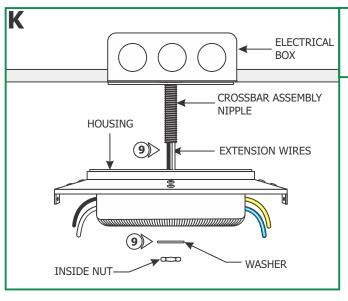
9: Feed the extension wires through the transformer housing center hole. Slide the transformer housing onto the crossbar assembly nipple and secure it in place by tightening the washer and inside nut.
