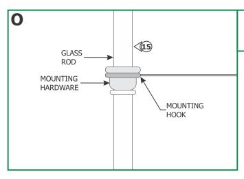
15: Carefully install the glass rods by seating them into the mounting hooks. Ensure the mounting hardware is fully seated in the mounting hooks.
