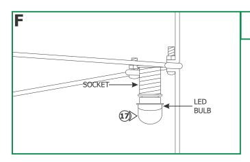
Install LED bulbs into each socket (MAX .5W 12VAC LED lamps)
