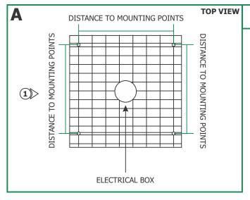
**1:** Measure the distance between the mounting points of the fixture. Make sure the electrical box is in the middle.
