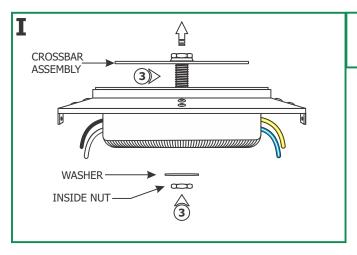
**3:** Remove the inside nut and washer to remove the crossbar assembly. **DO NOT DISASSEMBLE THE CROSSBAR ASSEMBLY.**
