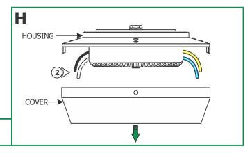
**2:** Unhook the transformer cover from the set screw and remove it from the transformer housing.
