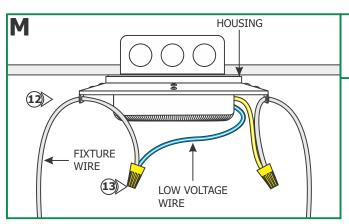
**12:** Feed each fixture wires through the side connectors.
