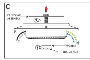
3: Remove the inside nut and washer to remove the crossbar assembly. <u>DO NOT DISASSEMBLE THE CROSSBAR</u> <u>ASSEMBLY.</u>
