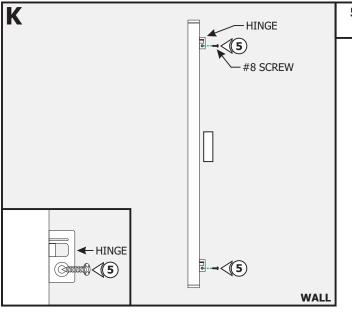
**5:** Line up the hinge to the anchors and secure it by tightening the #8 screws to each hinge.
