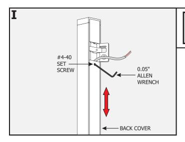
**NOTE:** If junction box is located at one end of the channel, then loosen the #4-40 set screw with the 0.05" Allen wrench on one of the back covers moving the opening hole to one end. Pull the wires out of that end & retighten the #4-40 set screw.
