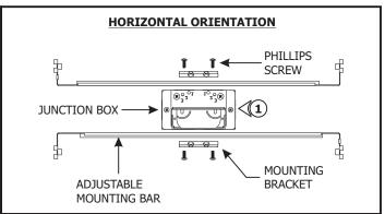
1: Mount each adjustable mounting bar to one side of the junction box (mounts to any side of the housing depending on the orientation of the channel) and secure them with the mounting brackets and two Phillips screws provided.
