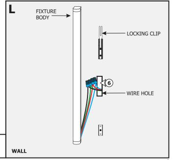
**6:** Refer to wiring diagrams on page 7 to connect the wires properly. Place all wire nut connections inside the junction box.
