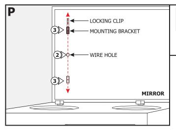
**NOTE:** Locking clip must be installed in the opposite direction of the fixture wire. Fixtures greater than 36" are provided with multiple locking clips.
