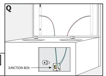
**NOTE:** (Optional) Junction box can be omitted for special installations or where permitted by local electrical code.
