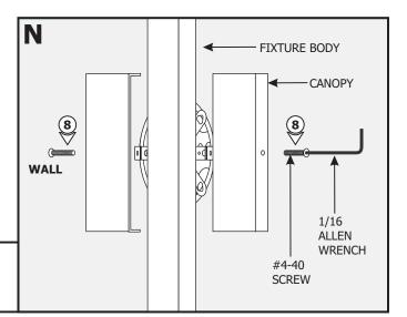
**8 (OPTIONAL):** For 4" Square Canopy installations, place each canopy piece against the crossbar and secure it to the electrical box holes with the provided #4-40 screws using the 1/16 Allen wrench.
