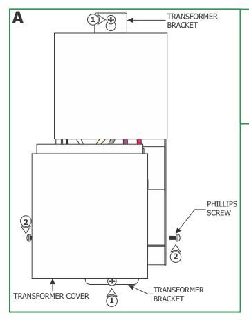
**NOTE:** In order to use small gauge wires from the transformer to the electrical box, it is recommended to install the remote transformers as near as possible to the electrical box. See "Low Voltage Wire Size Chart" on page 4.
