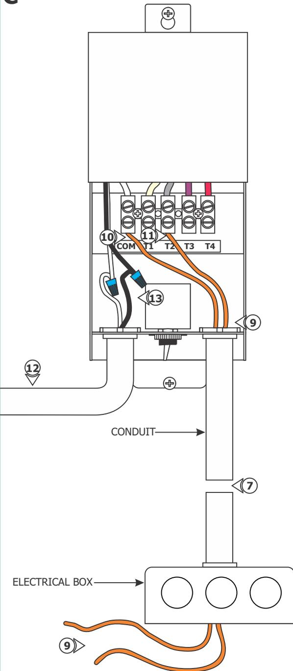
**7:** Install a conduit from the transformer to the electrical box.
