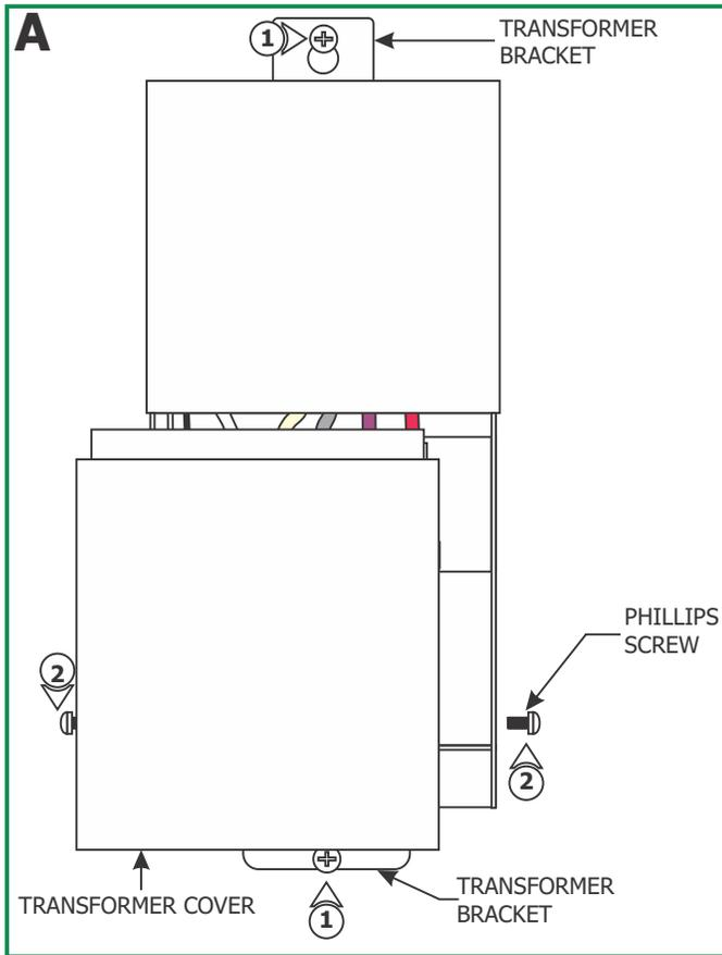
**NOTE:** In order to use small gauge wires from the transformer to the electrical box, it is recommended to install the remote transformers as near as possible to the electrical box. See "Low Voltage Wire Size Chart" on page 4.
