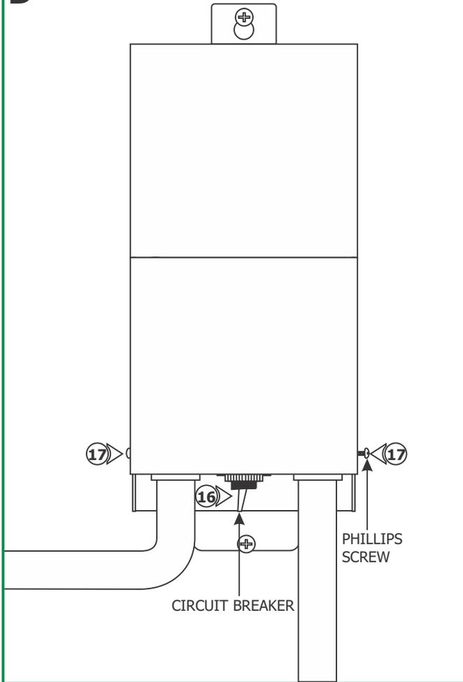
**14:** After installing the entire low voltage system, if the lamps have low intensity, then measure the voltage at the fixture closest to the power feed contacts with a voltmeter. The system must be at least 80% loaded and the voltmeter should read between 11V-12V ~AC. If the voltage does not fall in this range, call Edge Lighting "Technical Support" at 773-770-1195.
