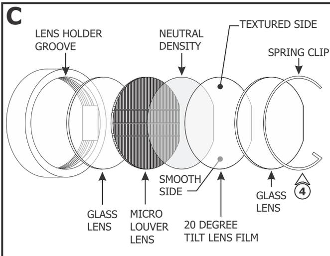
**3:** Carefully remove the spring clip and one of the glass lenses.
