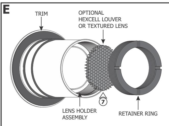
**7:** Place one optional Textured Glass (soft focus, linear spread etc) or Hexcell Louver (to reduce the glare) inside the retainer ring. **DO NOT USE** Hexcell Louver with Micro Louver together. Replace and tighten the retainer ring to secure the lens holder assembly in place.
