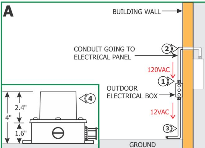
**NOTE:** If using a magnetic remote transformer to power the fixture omit the steps below and refer to the "Outdoor Installation Using Magnetic Remote Transformer" section.
