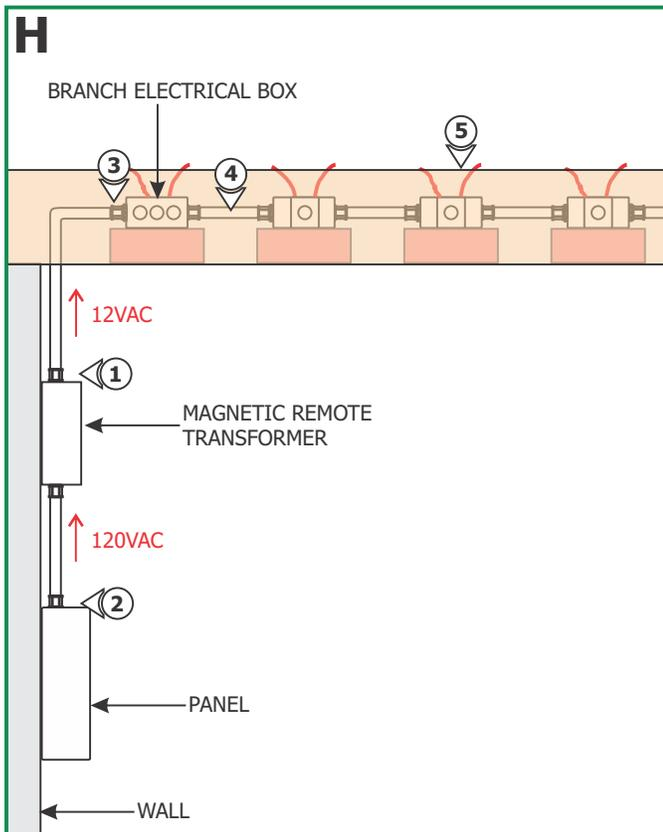
**1:** Install the magnetic remote transformer to an accessible location.
