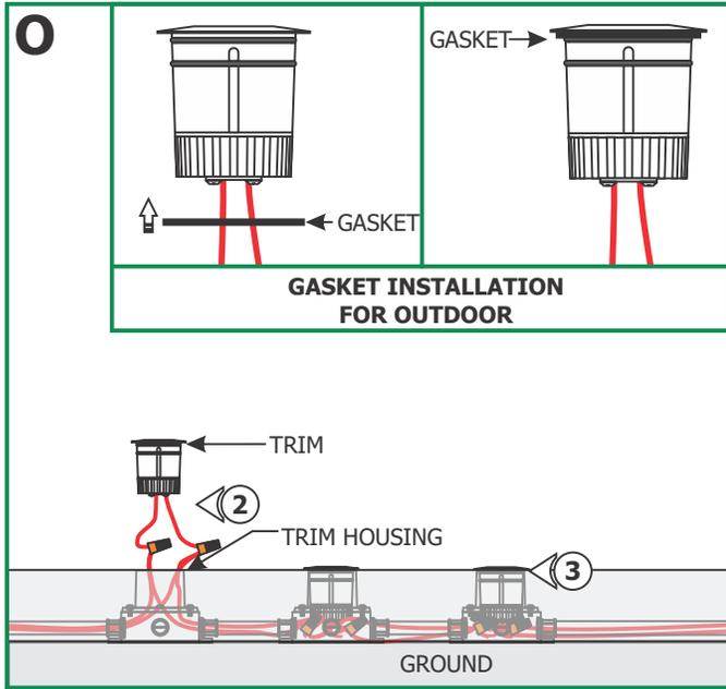
**NOTE:** If using the SUN3-LL accessory, refer to the instruction provided with the SUN3-LL to install the beam control accessories in each trim prior to wiring the trims.
