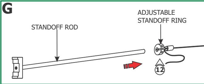
**12:** Slide the adjustable standoff ring onto the standoff rod. Make sure it passes mid point of the standoff rod.
