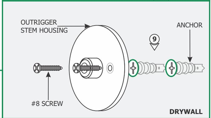
**8:** Mount the aircraft cable post integrated washer-nipple to the anchor using the #8 screw provided.
