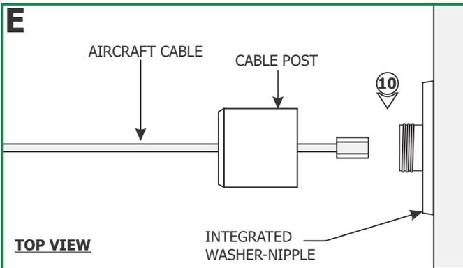
**10:** Feed the aircraft cable through the cable post and screw the cable post completely onto the integrated washer-nipple.
