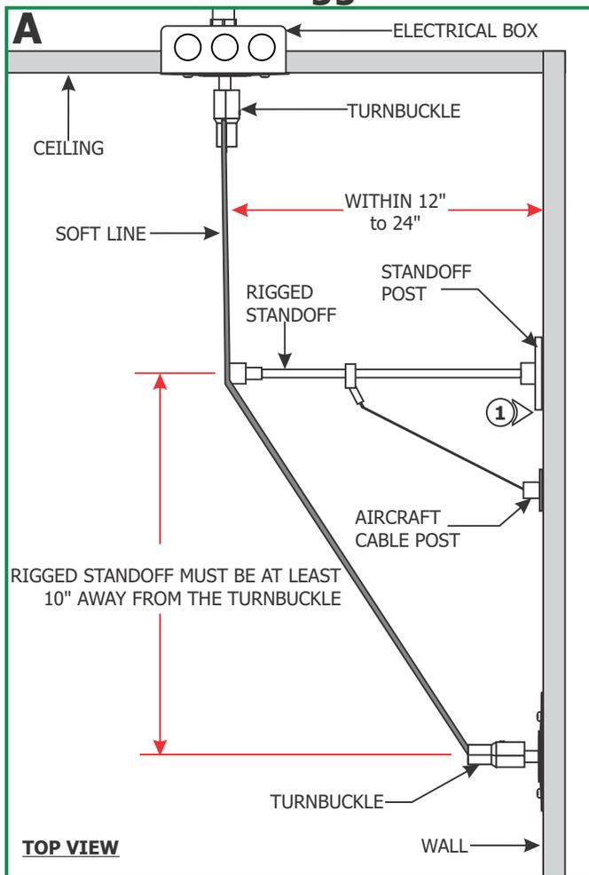
**NOTE:** This installation instruction should be used concurrently with Soft Line turnbuckles.
