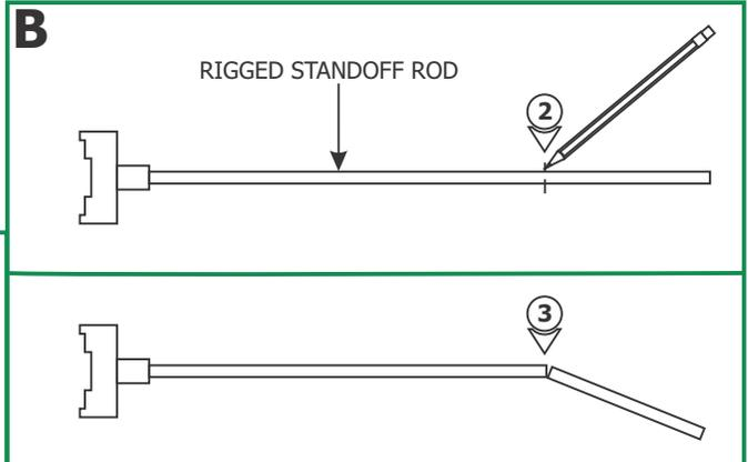
**2: Optional:** from the end of the rigged standoff rod, mark the point where the standoff rod needs to be shortened (minimum 12").
