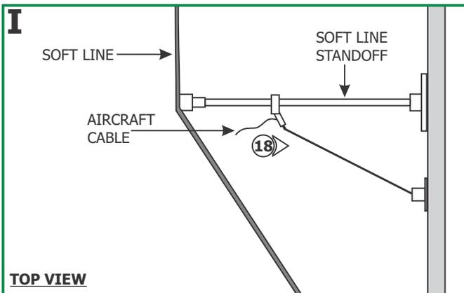
**18:** Pull the aircraft cable on all the soft line standoffs taut so that the standoff rods are all straight before tightening the turnbuckle adjustments links (refer to the turnbuckle instructions).
