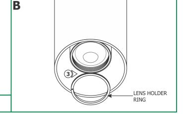
**3:** Replace and tighten the lens holder ring with the Allen wrench.
