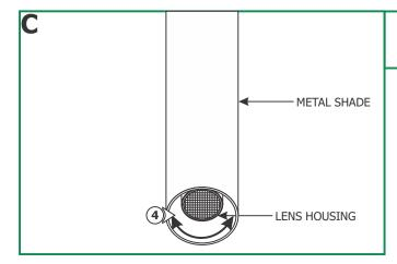
**4:** From the bottom of the metal shade rotate the lens housing to set the beam spread at either the spot or flood beam settings.
