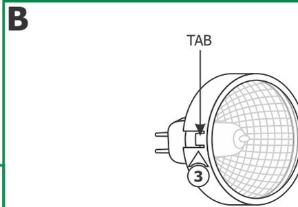
**3:** Press the tabs on the sides of the louver lens holder against the MR16 lamp to keep it in the position.
