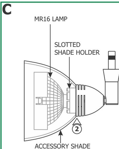
**1:** Place the MR16 lamp into the accessory shade and line up the MR16 lamp pins with the socket holes.
