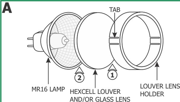
**1:** Place the Hexcell louver (Optional) or glass lens (Optional) or a combination of a hexcell and glass lens into the louver lens holder.
