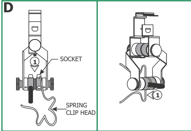
**1:** Push the spring clip completely onto the center of the socket groove until it snaps into place.
