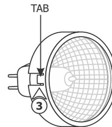
**3:** Press the tabs on sides of the snap lens holder against the MR16 lamp to keep it in the position.
