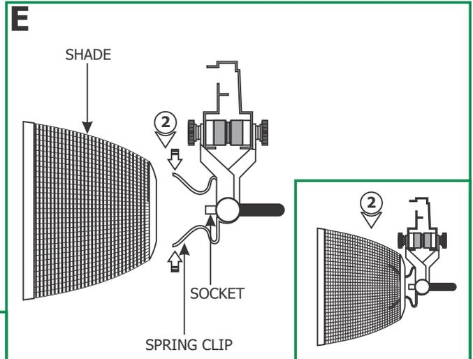
**2:** Squeeze the spring clip ends while inserting it into the shade.
