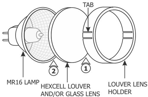
**1:** Place a Hexcell louver (Optional) or a glass lens (Optional) or a combination of a hexcell louver and glass lens into the louvers lens holder.
