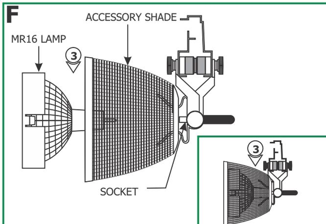
**3:** Place the MR16 lamp into the accessory shade and line up the MR16 lamp pins with the socket holes. Push the lamp pins completely into the socket holes.
