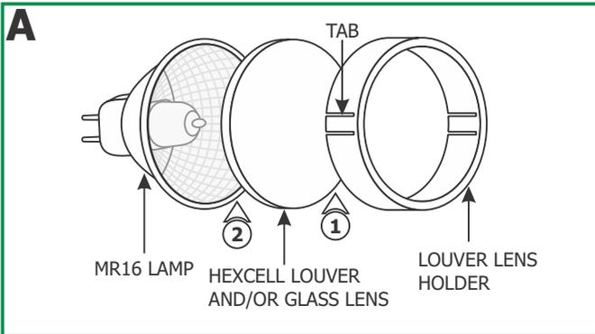
**1:** Place the Hexcell louver (Optional) or glass lens (Optional) or a combination of a hexcell and glass lens into the louver lens holder.
