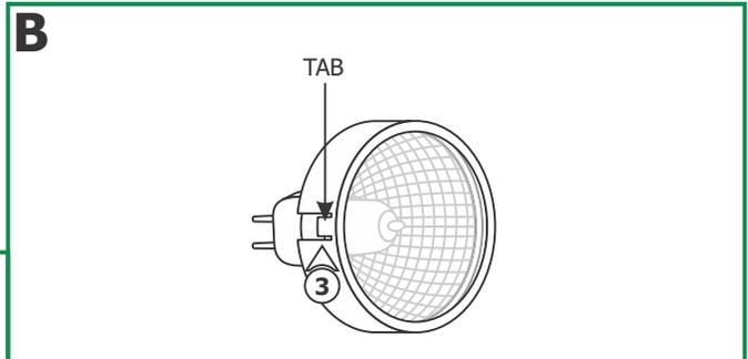
**3:** Press the tabs on sides of the snap lens holder against the MR16 lamp to keep it in the position.
