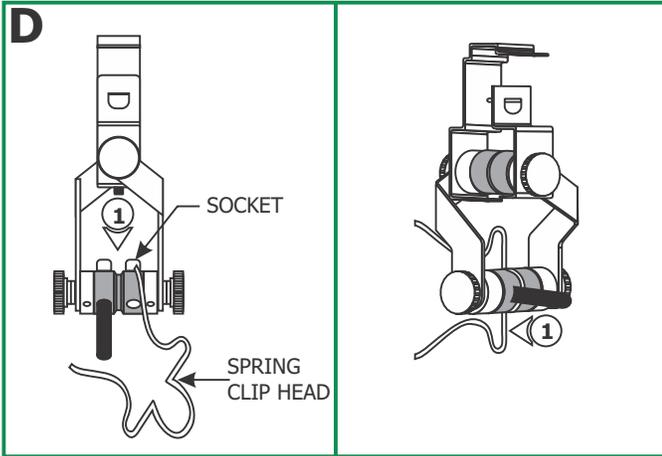
**1:** Push the spring clip completely onto the center of the socket groove until it snaps into place.
