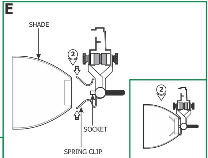
**8:** Squeeze the spring clip ends while inserting it into the shade.
