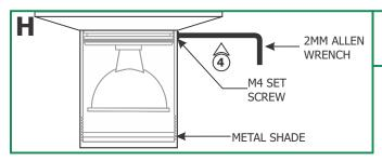
**4:** Push the metal shade completely onto the canopy and secure it in place by tightening the M4 set screw with the 2mm Allen wrench.
