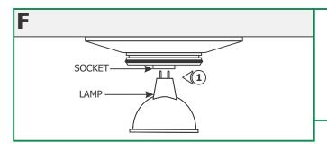
**CAUTION:** To reduce risk of a burn or electrical shock during lamping, disconnect the power to the fixture.
