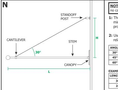
**NOTE:** Omit this section if the stem length is 14" and less and no cantilever is used (ceiling applications).
