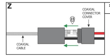
**15:** Replace the coaxial connector cover and tighten into place.
