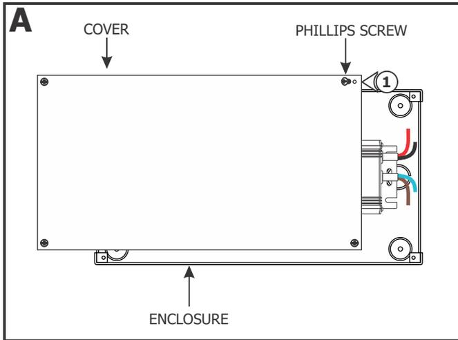
**1:** Loosen and remove the four Phillips screws on the front of the power supply cover to remove the cover from the enclosure.
