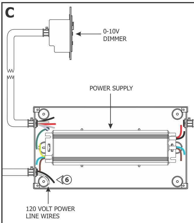
**6:** Run the 120 volt power line wires from the panel to the power supply enclosure.
