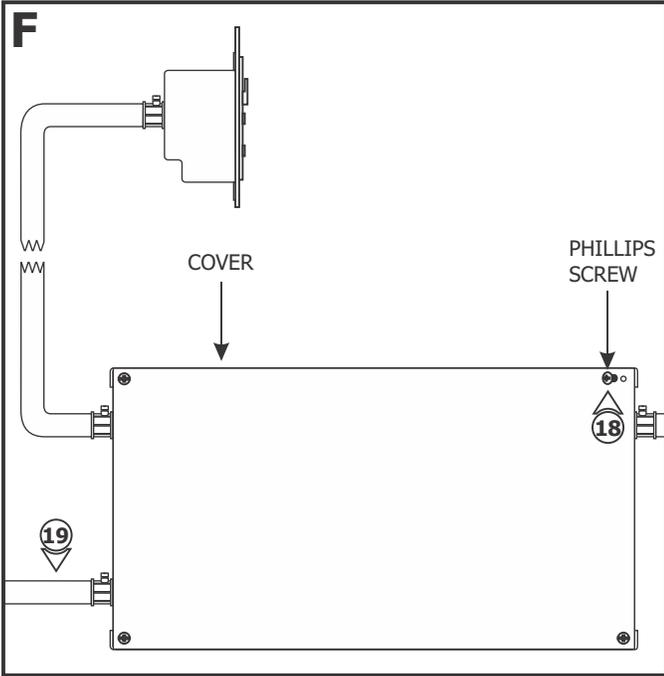
**18:** Replace the power supply cover and secure it by tightening the four Phillips screws.
