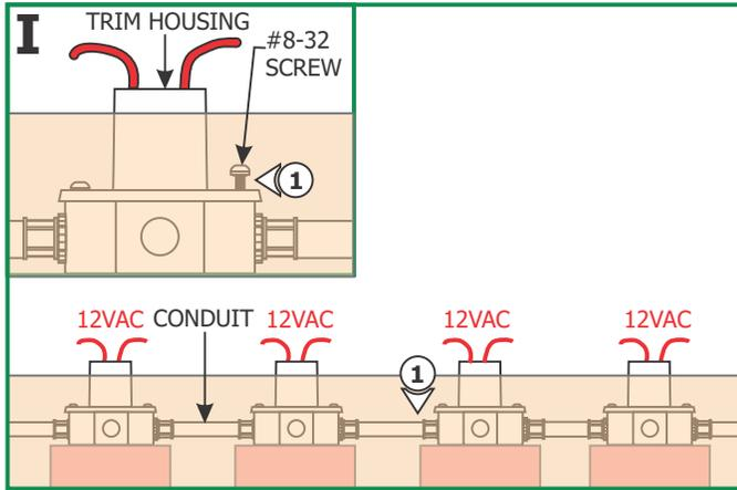
**1:** Align and secure the each trim housing to the octagon electrical box holes with the two #8-32 screws (not provided).
