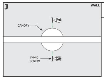
**20:** Align the canopy holes with the crossbar holes and secure the fixture to the crossbar with the provided #4-40 screws using a 1/16" Allen wrench.
