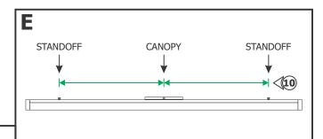
10: Measure the distance between the center of the canopy and each standoff post. Mark the locations of the standoff posts on the wall from the center of the junction box.
