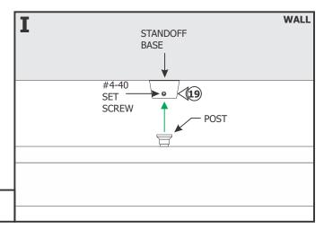
**19:** Align the posts on the fixture with the standoff bases and secure with the #4-40 set screws.
