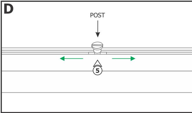
**5:** If necessary, adjust the position of the standoff post by loosening the post and sliding it across the channel. Tighten the post to secure in place.
