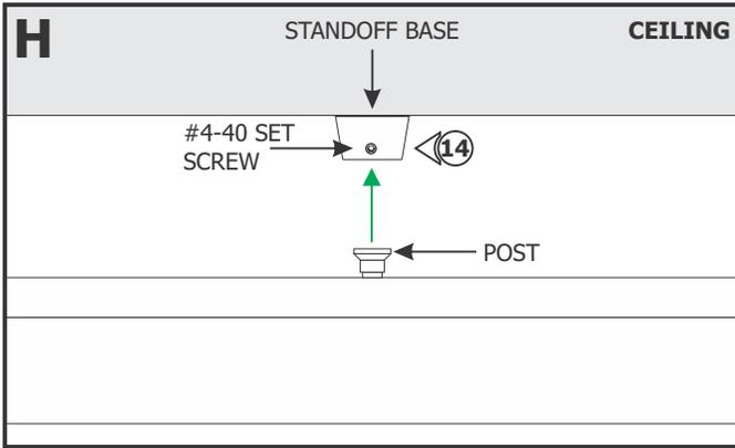
**14:** Align the post on the channel with the standoff base and secure with the #4-40 set screw using a 0.05" Allen wrench.
