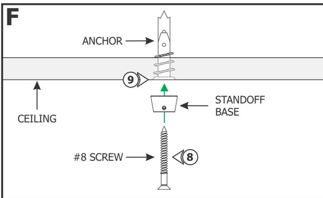
**8:** Feed the #8 screw through the standoff base into the anchor.
