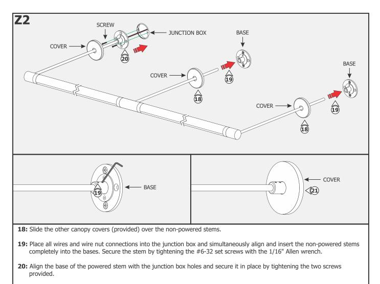
21: Slide the covers over the bases. The magnets on the back of the cover will keep the canopy in place.
