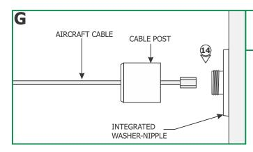
**14:** Feed the aircraft cable through the cable post and screw the cable post completely onto the integrated washer-nipple.
