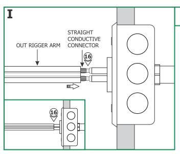
**16:** Push the out rigger arm entirely onto the straight conductive connectors, and hold it in place.
