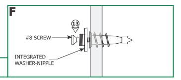
**13:** Mount the integrated washer-nipple to the anchor using the #8 screw provided.
