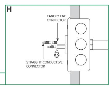
**15:** Push the straight conductive connectors into the canopy end connector.
