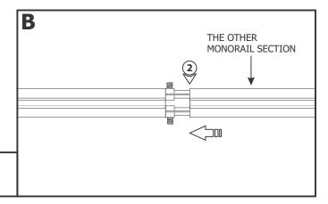
**2:** Push the other Monorail section entirely onto the straight isolating connectors and simultaneously connect the Monorail to the standoffs.
