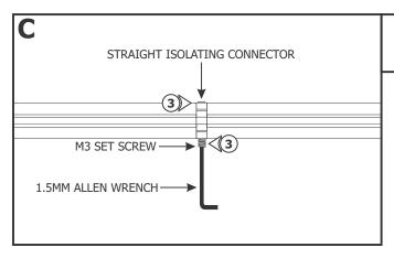
**3:** Tighten the M3 set screw on each of the isolating connectors firmly with the 1.5mm Allen wrench. **Do not over tighten** the set screws as this may strip the threads.
