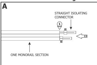
1: Push the straight isolating connectors completely into one Monorail section end. Make sure this Monorail section is secured with the standoffs (Refer to the instructions provided with the standoffs).
