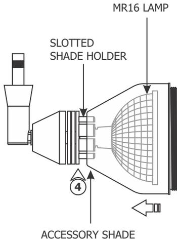
**3:** Line up the MR16 lamp pins with the socket holes.
