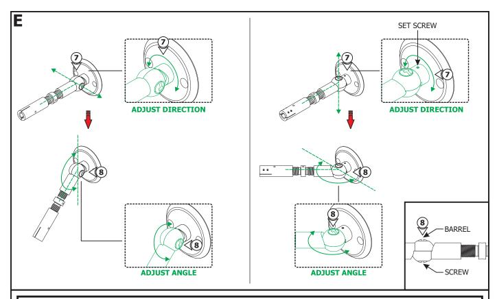
**NOTE:** The turnbuckle rotates around the canopy to adjust the direction and swivels at the base to adjust the angle of the Lazer Line.
