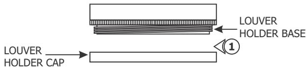
**1:** Unscrew and remove the louver holder cap from the louver holder base.
