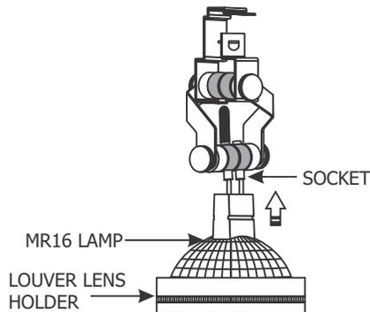
**5:** Push the lamp pins completely into the socket holes.
