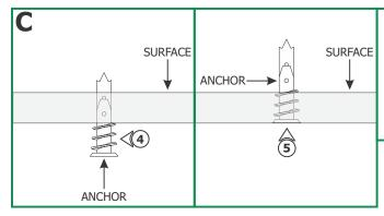
**NOTE:** Steps 4 through 6 are for drywall mounting. Omit these steps if mounting the clips to a wood surface directly.
