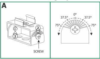
**3:** Place the mounting clips on the surface every 1' (measure from the the center of the mounting clip) and mark the screw locations.
