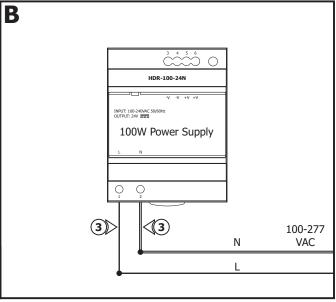
**3:** Connect the line power supply wire to the line voltage wire. Connect the neutral power supply wire to the line voltage neutral wire.
