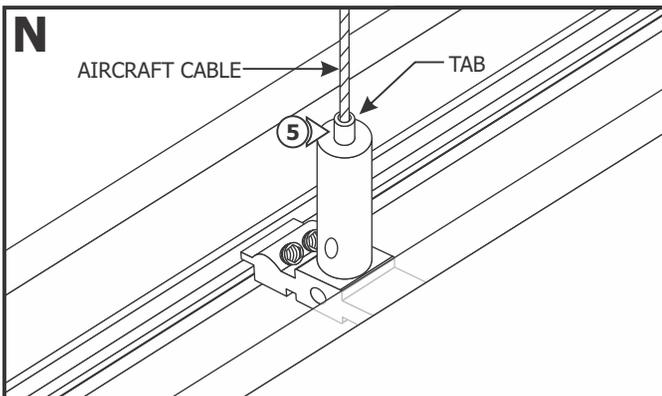
**5:** Insert the aircraft cable through the top of the tab on the sliding post.
