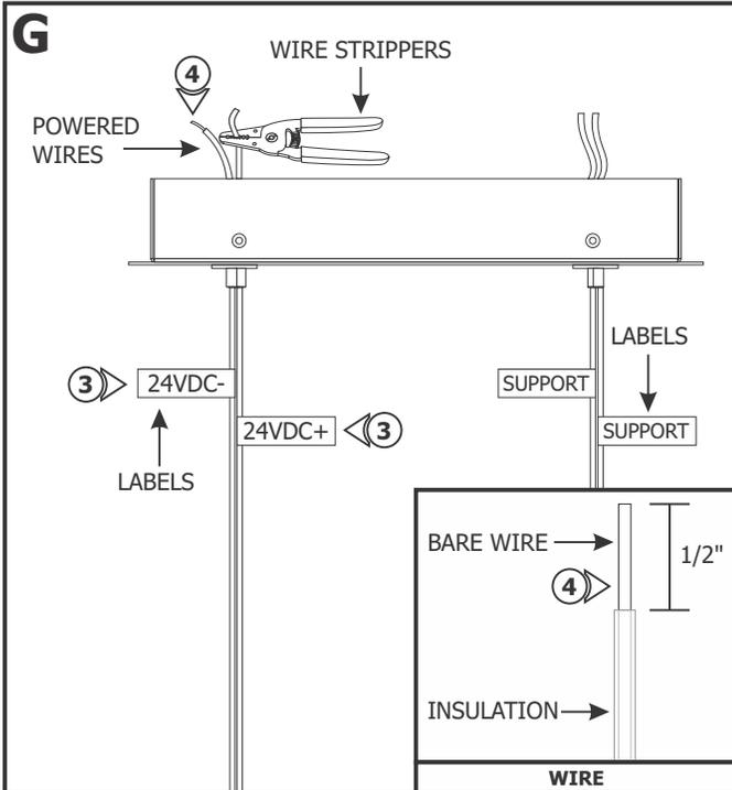
**NOTE:** The wires with "SUPPORT" labels are the support wires. **DO NOT** strip and power the support wires.
