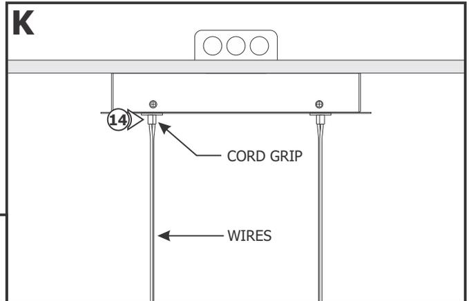
**14:** To make any adjustments to the fixture height, push the cord grips to slide the fixture up and down until the desired height is achieved. Release the cord grips to lock the wires in place.
