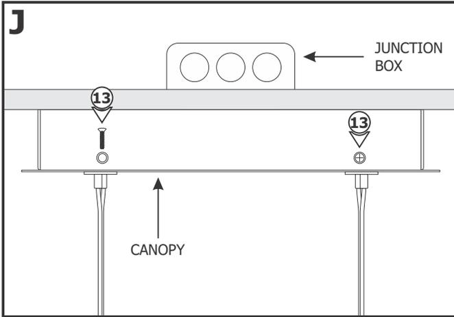
**12:** Place all the wires and wire nut connections inside the canopy.
