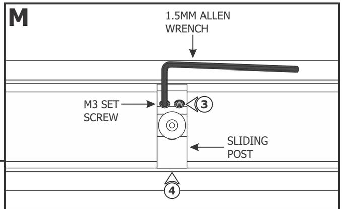
**3:** Tighten the two M3 set screws.
