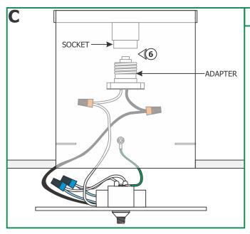
**6:** Screw the adapter completely into the medium base socket.
