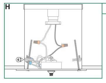
**6:** Screw the #10-24 long screws into the center hole of brackets.
