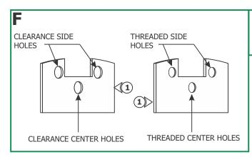
1: There are four mounting brackets included in the package, two of them with threaded holes and two others with clearance holes. Each set uses a threaded and a clearance hole brackets.
