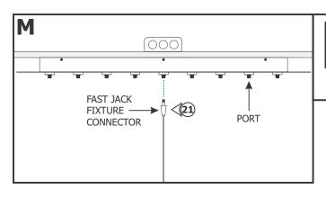
**CAUTION: Maximum** load of each port is **20** Watt. Use only fixtures that are rated 20 Watt or less, or relamp each fixture with a **Maximum 20** Watt lamp.
