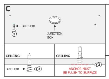
**NOTE:** Step 3 is for drywall mounting only. Omit these steps if mounting the canopy to a wood surface directly.
