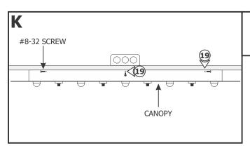
**18:** Place all wires and wire nut connections inside the canopy.
