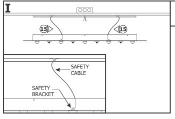
**15:** Feed one end of the safety cable into the safety bracket on the mounting plate. Insert the other end into the safety bracket on the canopy. Repeat for the other safety cable.
