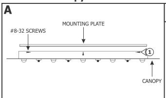
**1:** Remove the six #8-32 screws around the canopy to remove the mounting plate.
