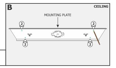
**2:** Align the mounting plate with the junction box. Using the mounting plate as a template, mark four mounting holes onto the ceiling.
