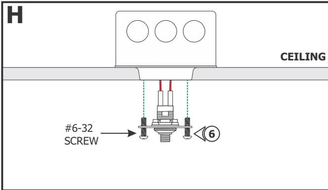
**6:** Place all wires and wire nut connections properly inside the electrical box. Mount the Fast Jack Port assembly to the 2" Plaster Ring using two #6-32 screws provided.
