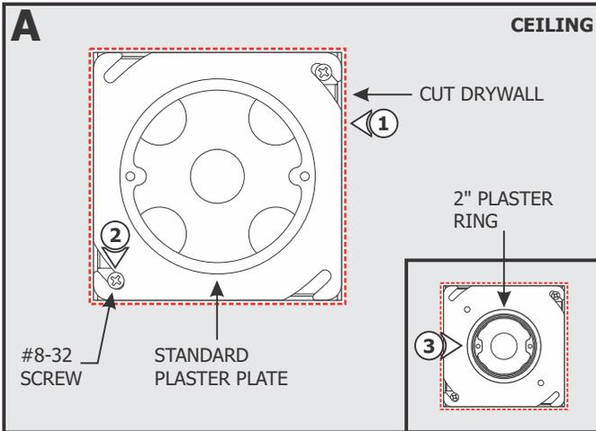
**NOTE:** Electrical box must be minimum 2.2" deep. Otherwise refer to Section Two to install the provided 2.2" deep electrical box with hanger bars.
