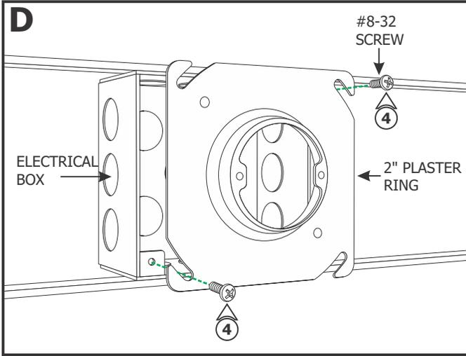
**NOTE:** Electrical box must be mounted to allow clearance of 1/2" between the face of the junction box and the drywall surface.
