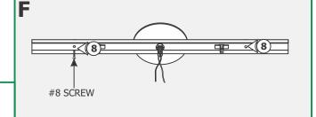
**8:** Secure the mounting plate to the anchors with the provided #8 screws.
