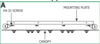
**1:** Remove the sixteen #8-32 screws around the canopy to remove the mounting plate.
