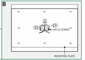
**NOTE:** It is recommended that a person to hold the mounting plate while the electrician installs it.
