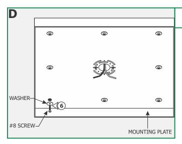
**6:** Secure the mounting plate to the anchors with the provided #8 screws and washers.
