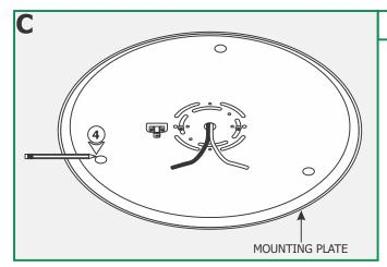
4: Mark the three mounting plate holes on the ceiling.
