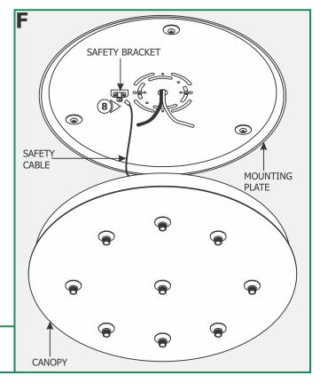
**8:** Insert one end of the safety cable into the safety bracket of mounting plate and the other end into the canopy safety bracket.
