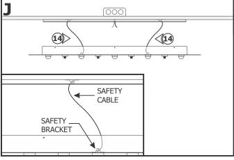
**14:** Feed one end of the safety cable into the safety bracket on the mounting plate. Insert the other end into the safety bracket on the canopy. Repeat for the other safety cable.
