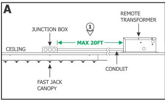
1: Run the low voltage wires from a remote transformer to the junction box where the Fast Jack canopy is going to be installed. It is recommended to install the remote transformer near the junction box to avoid voltage drop. Refer to the low voltage wire size chart provided with the remote transformer.
