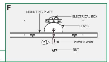
**7:** Slide the cover and mounting plate center hole onto the crossbar threaded nipple and secure it with the nut provided.
