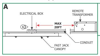
1: Run the low voltage wires from a remote transformer to electrical box where Fast Jack canopy is going to be installed. It is recommended to install the remote transformer near the electrical box to avoid voltage drop. Refer to the instructions provided with remote transformer for low voltage wire size chart. Refer to the low voltage wire size chart provided with the remote transformer.
