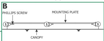
**1:** Loosen and remove the six Phillips screws from the canopy to remove the mounting plate.
