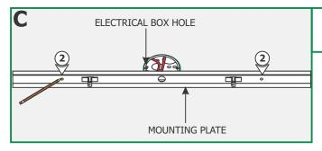
**2:** Align the mounting plate holes with the electrical box holes and mark a point through the mounting plate holes onto the ceiling. These points are used for the anchors.
