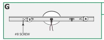
**8:** Secure the mounting plate to the anchors with the provided #8 screws.
