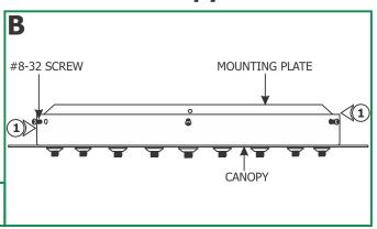
**1:** Loosen and remove the six #8-32 screws around the canopy to remove the mounting plate.
